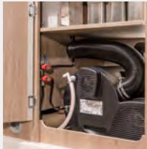
"TRUMA Combi 4E" gas heating (except TRAIL/BOX 200)
